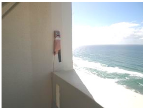
View of dust collection from a high rise building for chloride analysis.
