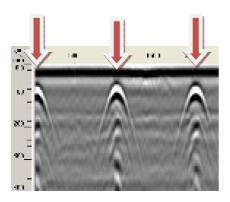
The image below shows several, live high voltage cables, entering the concrete slab. These can be traced using our high quality electromagnetic field detection unit.
