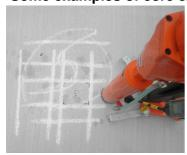
Compressive strength can be affected by embedded object in the core that has been extracted. It is ideal to perform GPR prior to core extraction to avoid reinforcement and other embedded objects that may affect the results.
